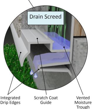
DRAIN SCREED is a vinyl HI-PERFORMANCE trim that provides a straight, true, continuous surface that terminates the base of a stucco wall. DRAIN SCREED integrates many features to simplify installation providing guides to help installers maintain the proper stucco thickness. The key feature is the vented moisture trough which allows rain screen to be inserted to maintain the drainage cavity throughout the wall and out the bottom.
